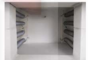
Furnace interior with high-quality fiber insulation
