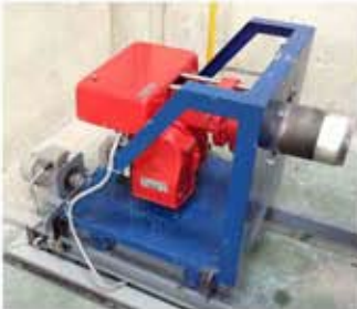
Two-Step gas burner for low-load and high-load mode
