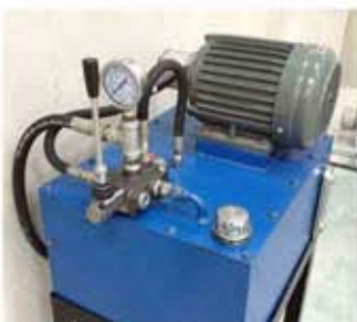
Hydraulics assembly with non-flammable hydraulic fluid
