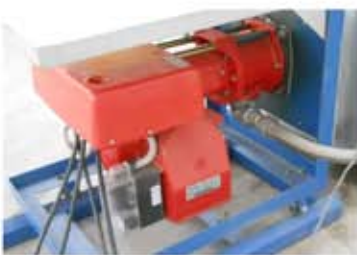
Two-Step gas burner for low-load and high-load mode
