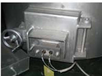
Emergency outlet for the safe draining of melting in case of crucible breakage
