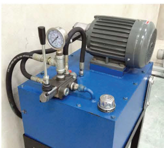
Hydraulics assembly with nonflammable hydraulic fluid
